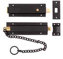
Cast brass and cast iron. Pull chain to release top bolt, lift handle to release foot bolt.
