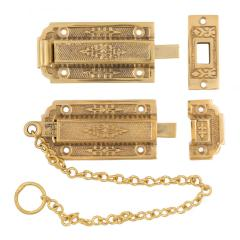
Cast brass and cast iron. Pull chain to release top bolt, lift handle to release foot bolt. For narrow stile doors.
