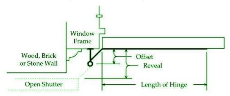
The length of strap hinges should be close to 3/4 of the width of the shutter.
